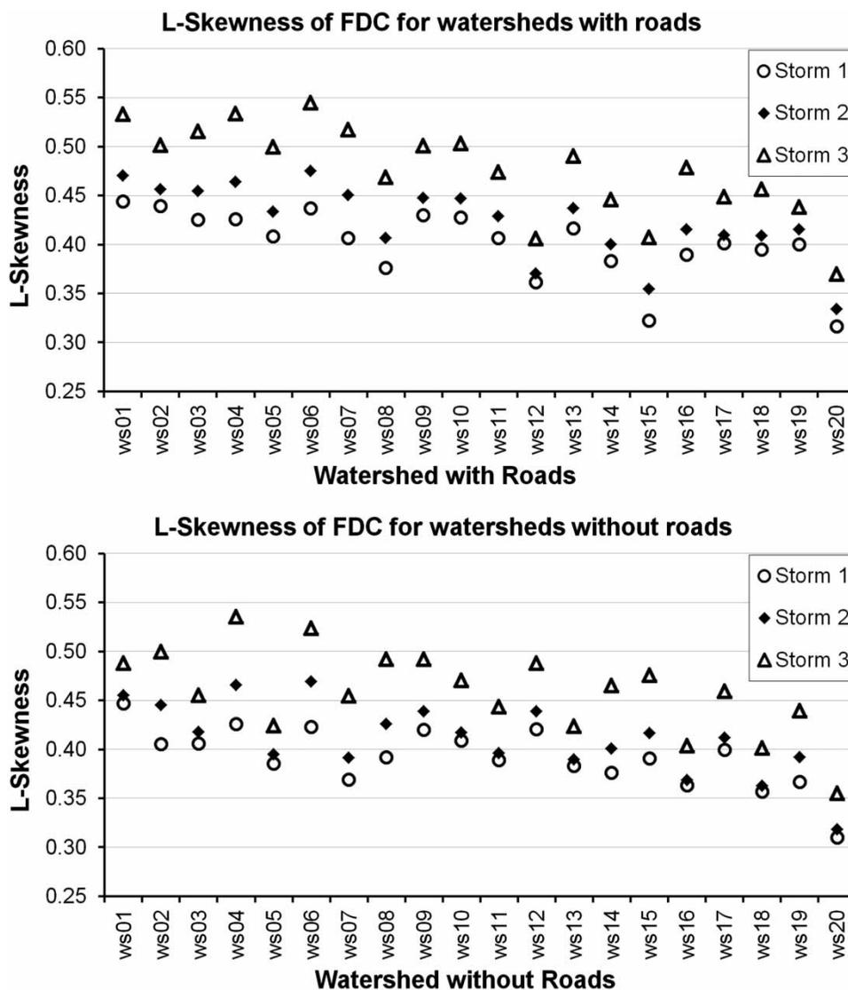
**Figure 6** | Linear skewness of the FDCs calculated for the watersheds with roads and without roads in the study area implementing three storms. Watersheds are sorted ascending by the area from 1 to 20.
