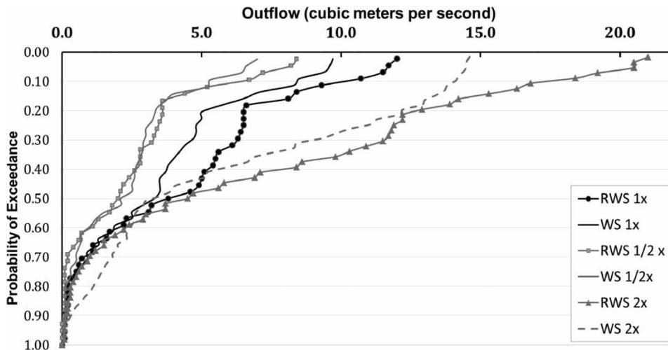
**Figure 4** | An illustration of FDC for one watershed (number 16) with and without roads showing the differences in percent of time flow was equaled or exceeded in response to three different storms. RWS stands for the watershed with road and WS stands for the watershed without roads; 1x, 1/2x, and 2x stand for storms with one, half, and double intensity, respectively.
