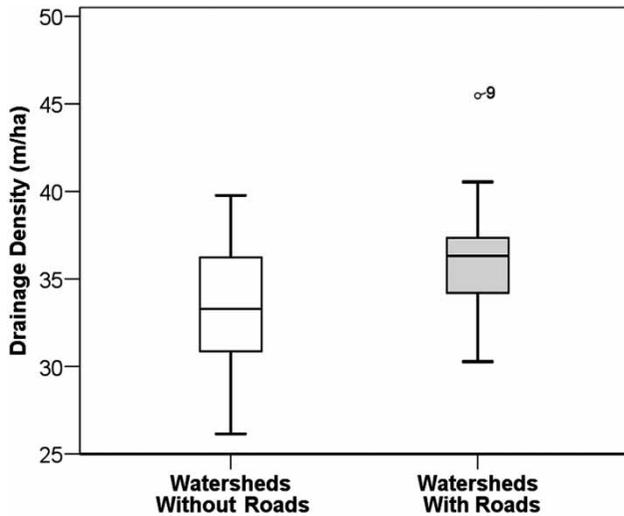
**Figure 8** | Box plot showing the measure of variation in drainage density for watersheds with roads and after removal of roads from the topography of the watersheds. Box, whiskers, and upper and lower edge demonstrate the interquartile range, 25% of data, and largest and smallest values that are not outliers, respectively. Values that are outside the box and whisker are outliers.
