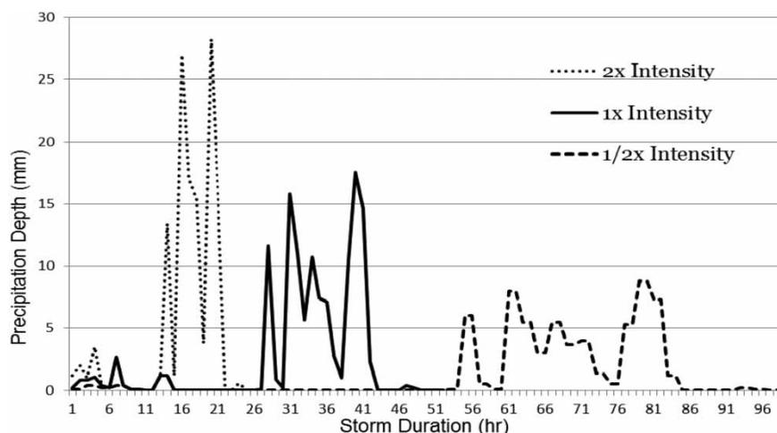
**Figure 2** | Three storms with different intensities implemented in the HEC-HMS model. The bold line is the original storm recorded on 4 August 2004. Dashed lines are design storms with half and double intensities.
