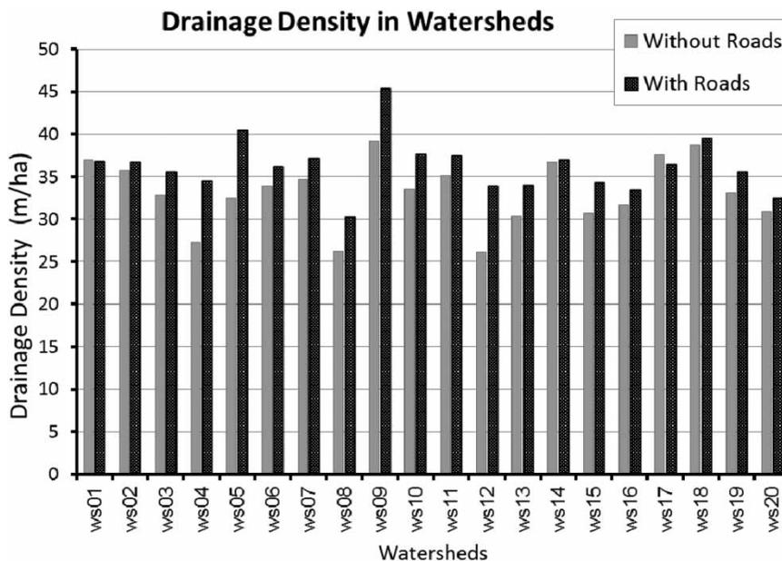
**Figure 5** | Comparison between drainage density before and after elimination of roads from the topography of the watersheds. Drainage density values are illustrated in black for watersheds with roads and in grey for watersheds after roads were removed. Watersheds are sorted ascending by the area from 1 to 20.
