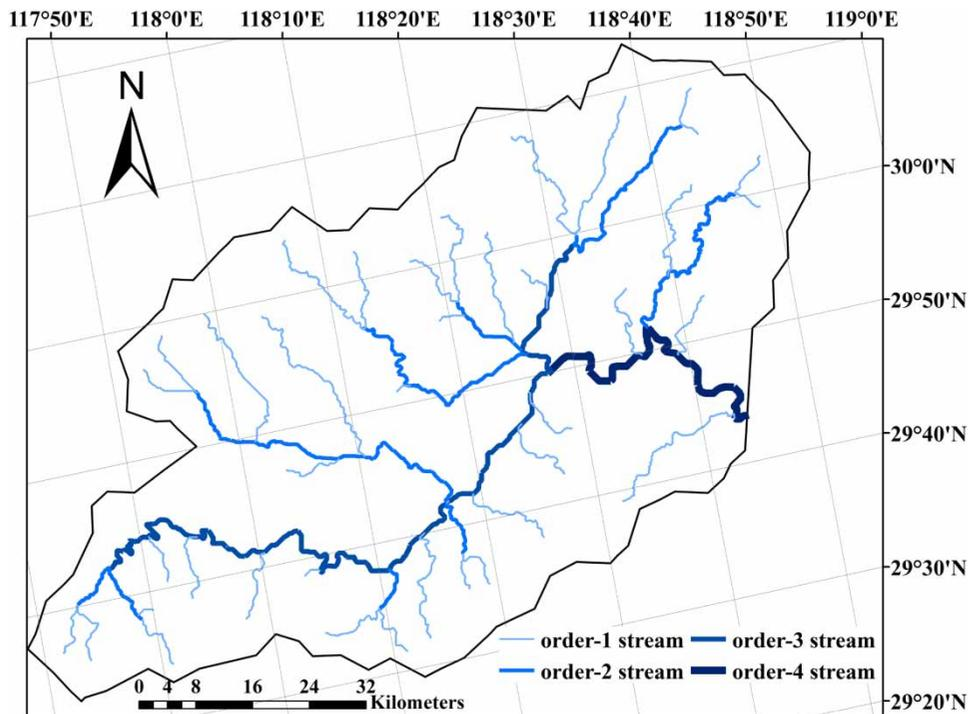
**Figure 3** | River networks of the study catchment ordered by the Horton–Strahler system.
