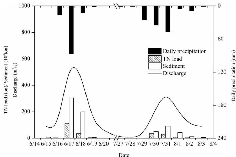
**Figure 11** | Comparison of daily TN load, sediment, and discharge during two rainfall events in 2008 at Yuliang station.
