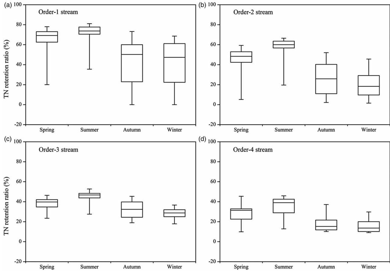
**Figure 9** | Seasonal variations of the average TN retention ratios in streams of different orders (box plots display 2.5th, 25th, 50th, 75th, and 97.5th percentiles).
