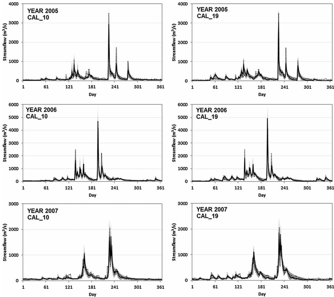
**Figure 4** | Comparison of simulated streamflow by behavioral parameter sets obtained from CAL\_10 and CAL\_19 for calibration period (2005–2007). Dashed lines: observed streamflow; gray band: 95% uncertainty band of ensemble simulation; solid lines: best simulation of ensemble prediction.
