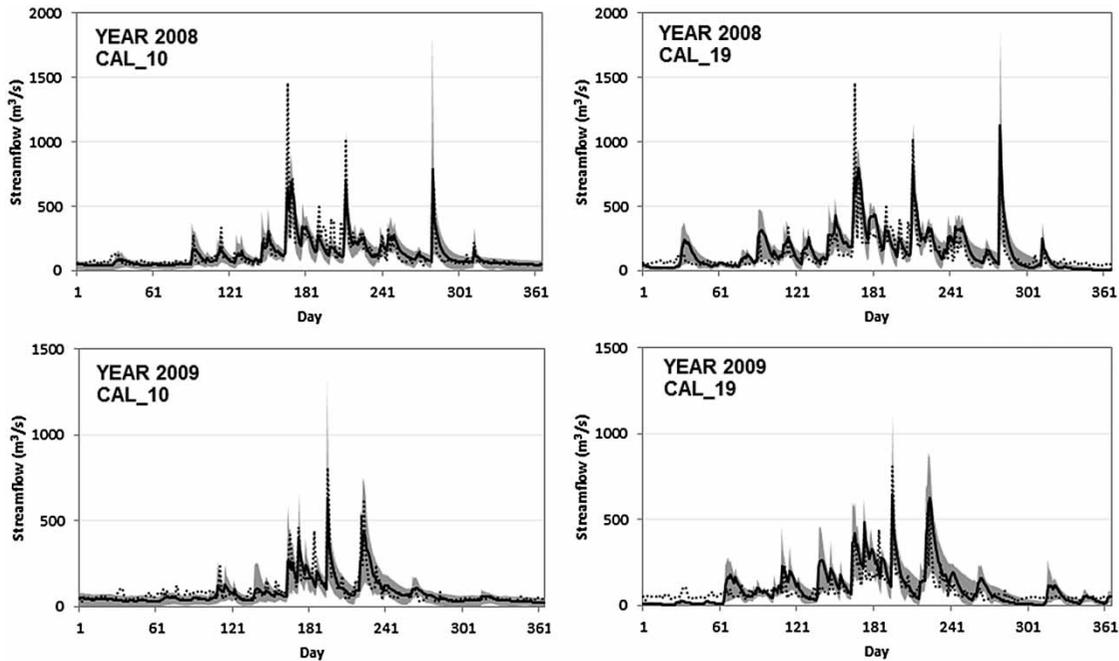
**Figure 5** | Comparison of simulated streamflow by the behavioral parameter sets obtained from CAL\_10 and CAL\_19 for validation period (2008–2009). Dashed lines: observed streamflow; gray band: 95% uncertainty band of ensemble simulation; solid lines: best simulation of ensemble prediction.
