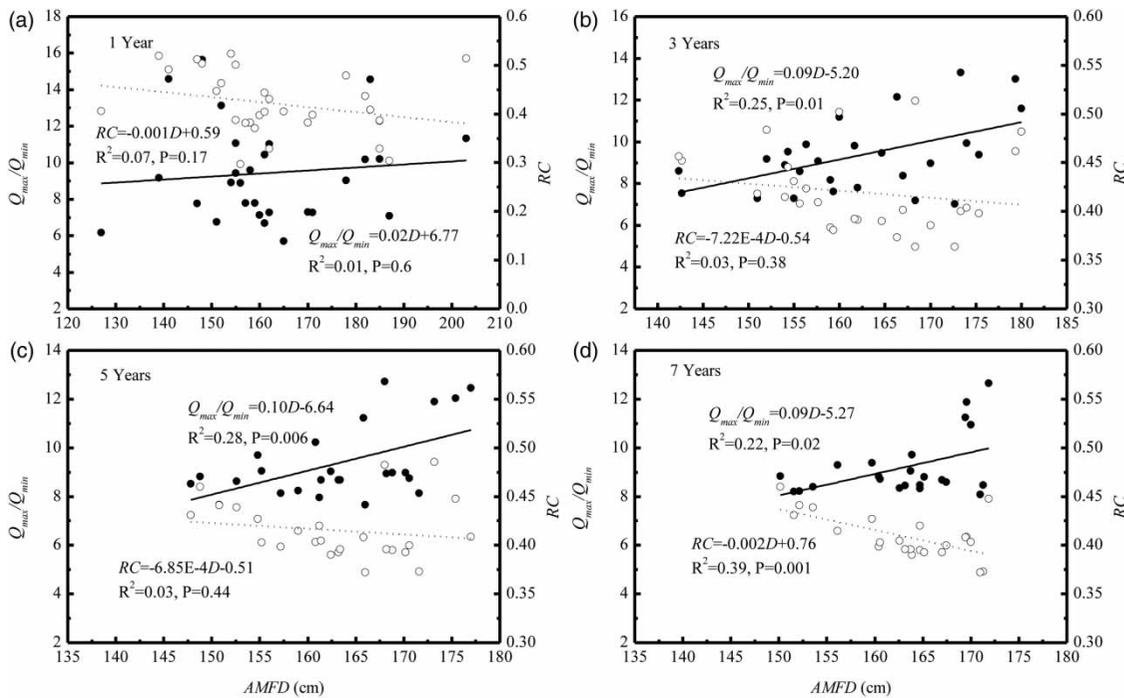
**Figure 8** | RC in winter vs. AMFD (solid circles and lines) and  $Q_{max}/Q_{min}$  vs. AMFD (open circles and dashed lines) based on the (a) 1-year, (b) 3-year, (c) 5-year and (d) 7-year moving average methods at the Tangnaihai Hydrometric Station.
