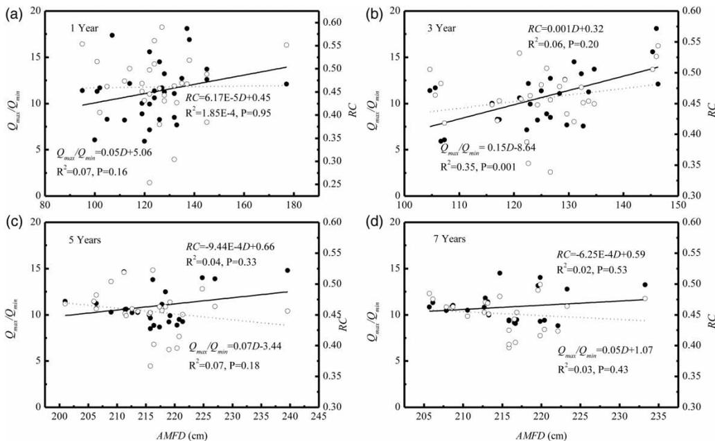
**Figure 7** | RC in winter vs. AMFD (solid circles and lines) and  $Q_{max}/Q_{min}$  vs. AMFD (open circles and dashed lines) based on the (a) 1-year, (b) 3-year, (c) 5-year and (d) 7-year moving average methods at the Maqu Hydrometric Station.
