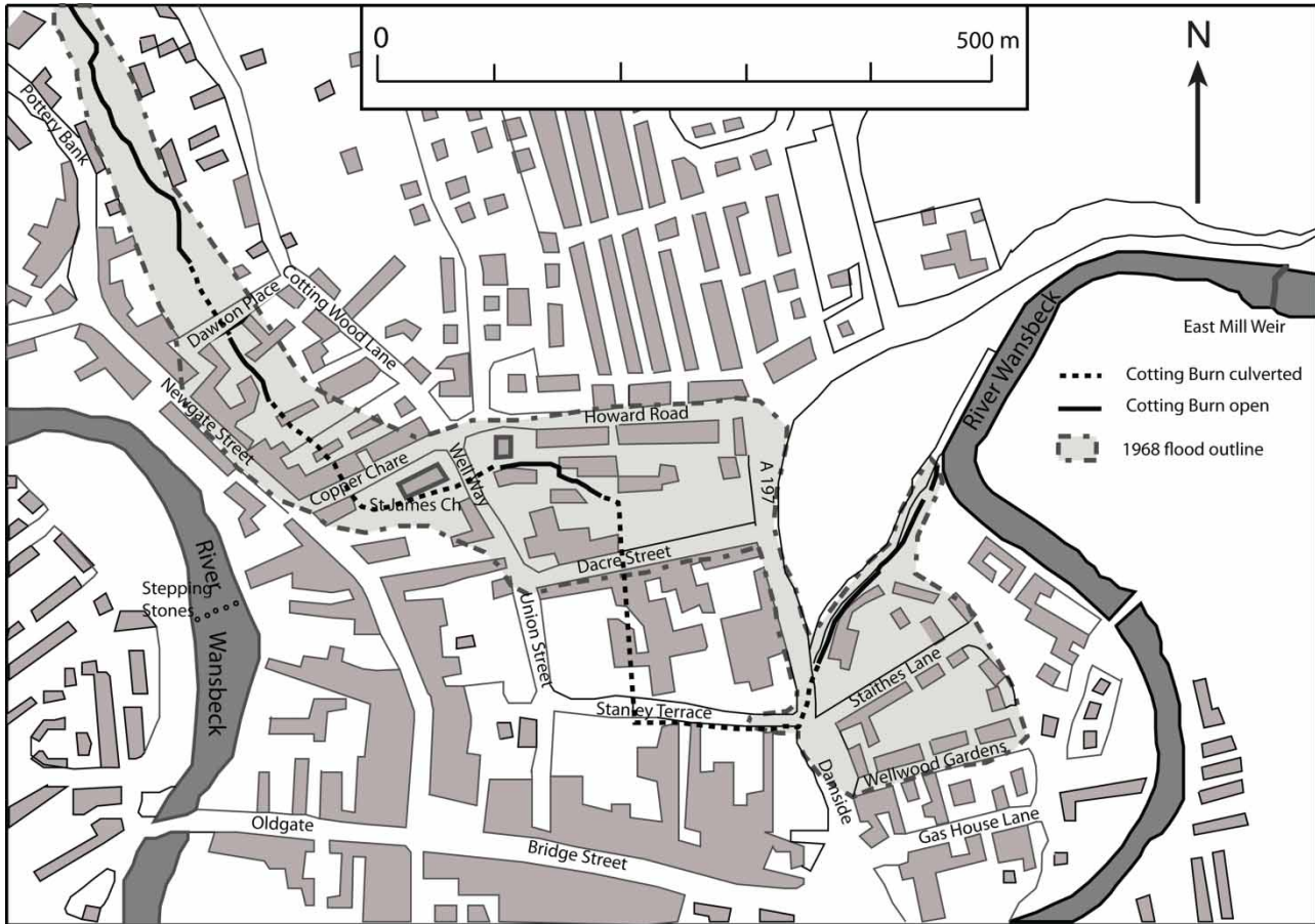
Figure 5 | Map of Morpeth showing the Cotting Burn flash flood extent in the event of September 1968.
