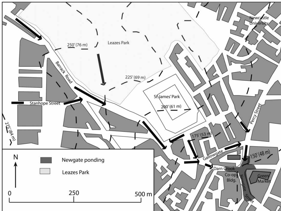
Figure 3 | Pathways of repeated surface water flow towards Newgate Street (bottom right) where ponding occurs.
