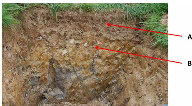
Figure 1 | Both Halstow and Hallsworth soil series at North Wyke have clay loam soil to 30 cm depth (soil horizons marked A) over a dense impermeable clay subsoil with coarse prismatic soil structure (soil horizons marked B). Photo shown is of a Hallsworth soil.
