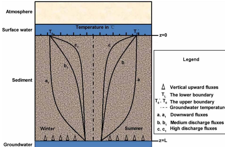
**Figure 4** | Schematic of vertical temperature profiles for one-dimensional heat and water transport in a streambed based on the thermal steady-state conditions in winter and summer seasons; a, b, c show the vertical water fluxes in summer; a<sub>1</sub>, b<sub>1</sub>, c<sub>1</sub> show the vertical water fluxes in winter (modified from Anibas et al. (2011)).
