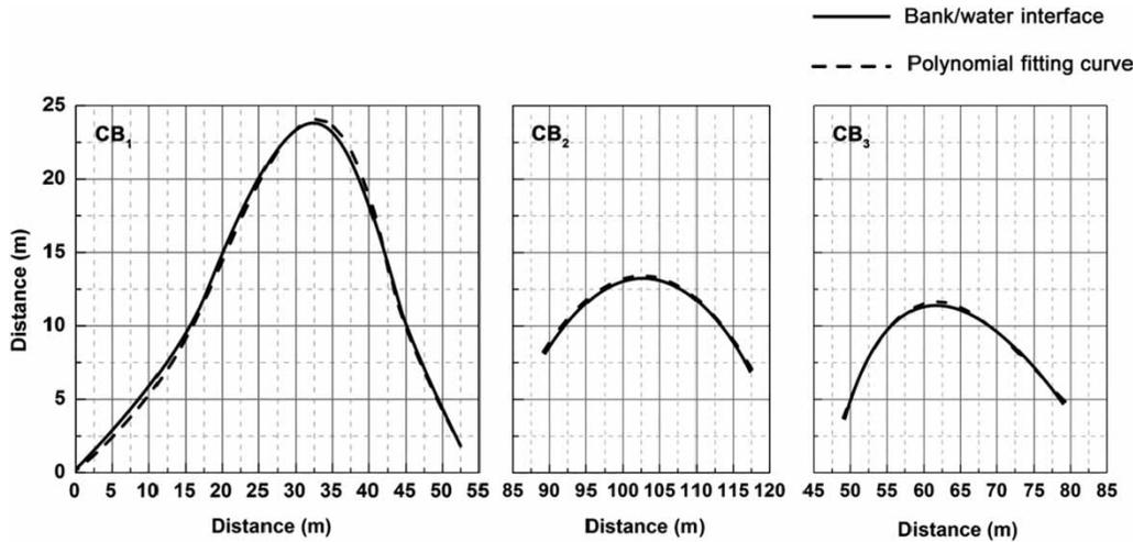
**Figure 5** | The polynomial fitting curves for two convex banks in January 2015 (CB<sub>1</sub>, CB<sub>2</sub>) and one convex bank in July 2015 (CB<sub>3</sub>). The solid line indicates the bank/water interface along the meandering banks; the dashed line indicates the polynomial fitting curve for the bank/water interface.
