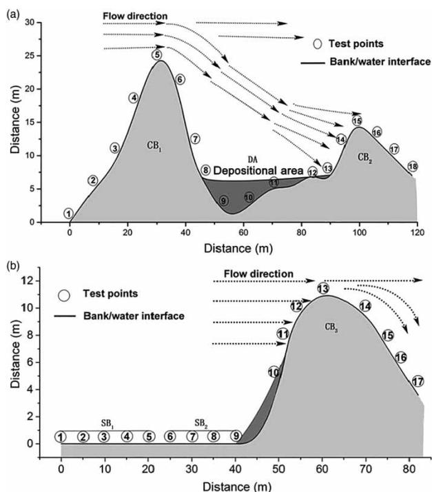
**Figure 3** | Test sites showing the three divided sections along the bank in January 2015 (a) CB<sub>1</sub>, AD, CB<sub>2</sub> and three other divided sections along the bank in July 2015 (b) SB<sub>1</sub>, SB<sub>2</sub>, CB<sub>3</sub>. (The x-axis is the distance from the first test point on the bank along the flow direction; the y-axis is the perpendicular distance from the test site point to the x-axis.)
