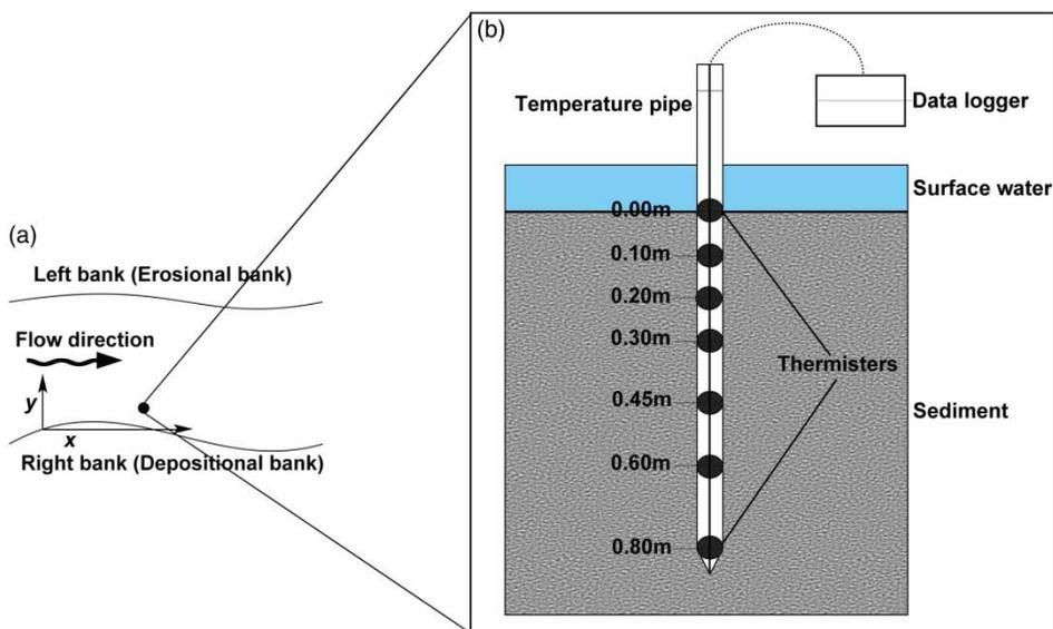
**Figure 2** | Schematic diagrams of the locations of test points close to the right bank in the Weihe River, indicating the sediment erosion and deposition along the bank (a), and measurement setup of temperature distributions in streambed sediment with the temperature pipe (b).
