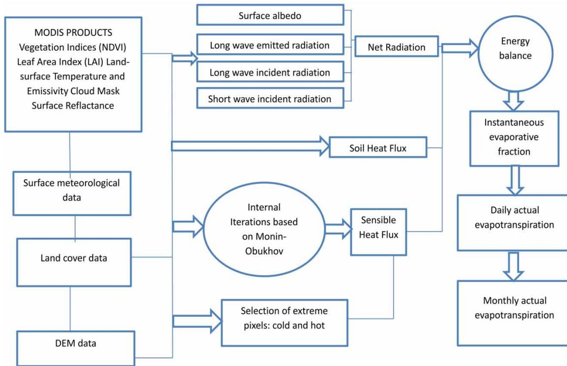
Figure 3 | Flowchart of ET estimation by using METRIC.
