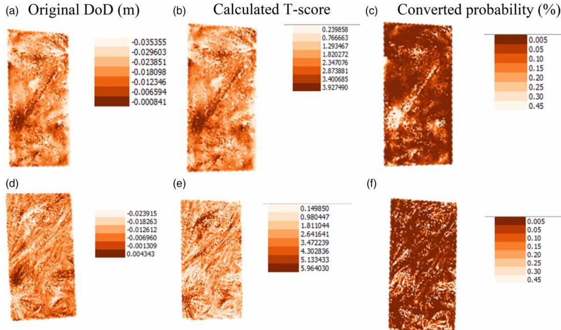
**Figure 4** | DEM of the differences (DoD) for SfM (a), t-score obtained from Equation (2) (b), cumulative distribution probability (c); DEM of the differences (DoD) for TLS (d), t-score obtained from Equation (2) (e), cumulative distribution probability (f).
