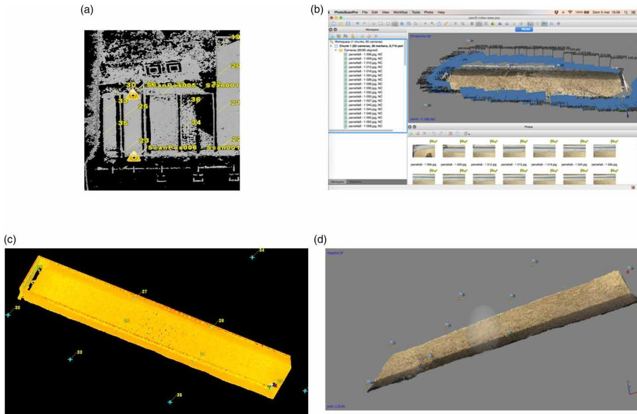
**Figure 1** | Positions of the TLS scans (represented by the triangle) and positions of 13 targets (GCPs) (a); scheme of alignment frames (b); model of the  $2 \times 11$  m plot obtained from the TLS survey (c); and dense point cloud model of the  $2 \times 11$  m plot obtained from the SfM survey (d).
