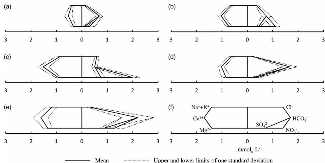
**Figure 7** | Stiff diagrams for the respective clusters with mean value and upper and lower limits of one standard deviation by obtained reference vectors: (a) cluster-1, (b) cluster-2, (c) cluster-3, (d) cluster-4, (e) cluster-5, and (f) legend.
