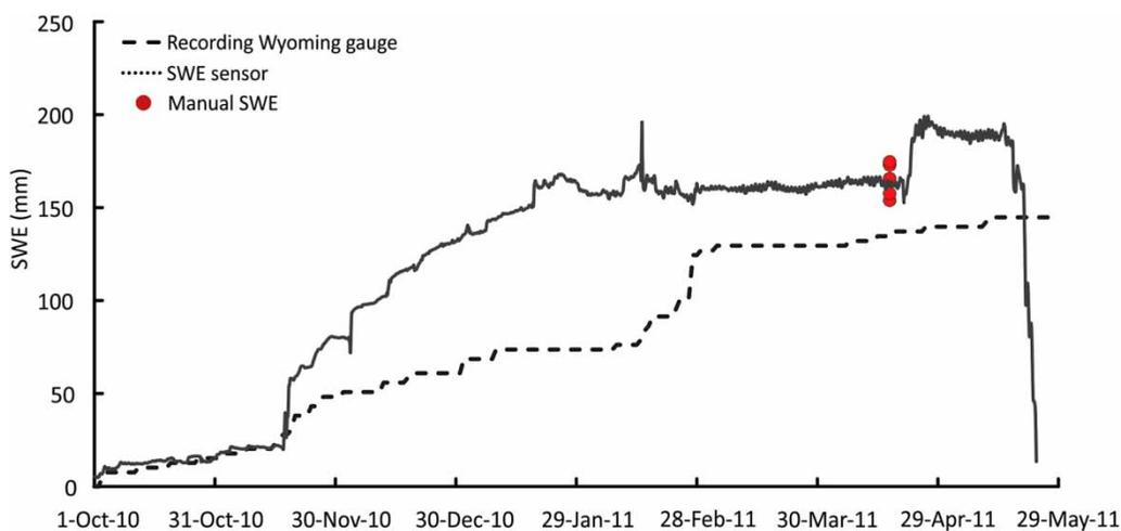
**Figure 5** | Cumulative winter snowfall measured by the NRCS recording precipitation gauge equipped with a Wyoming shield, SWE on the ground measured by the SWE sensor (grey line), and manual snow survey measured at the SWE sensor.
