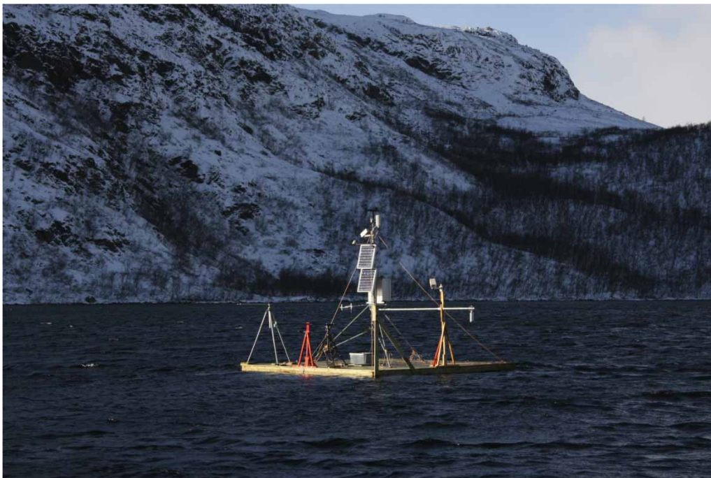
Figure 2 | Automated ice station Lotus in Lake Kilpisjärvi.
