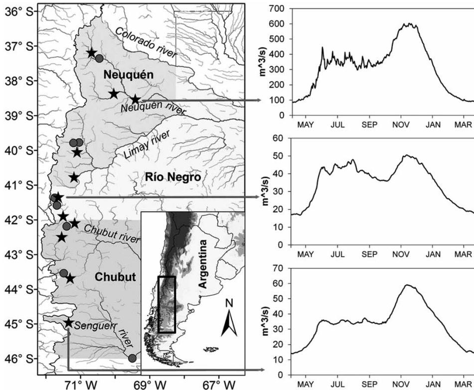
**Figure 1** | Location of the study area, the main rivers selected for this cycle, and the spatial distribution of the hydrological stations. Stations marked with a star were used for the climatology of streamflow droughts. The hydrological annual cycle is shown for three selected rivers (from north to south: Neuquén, Manso, and Senguerr).
