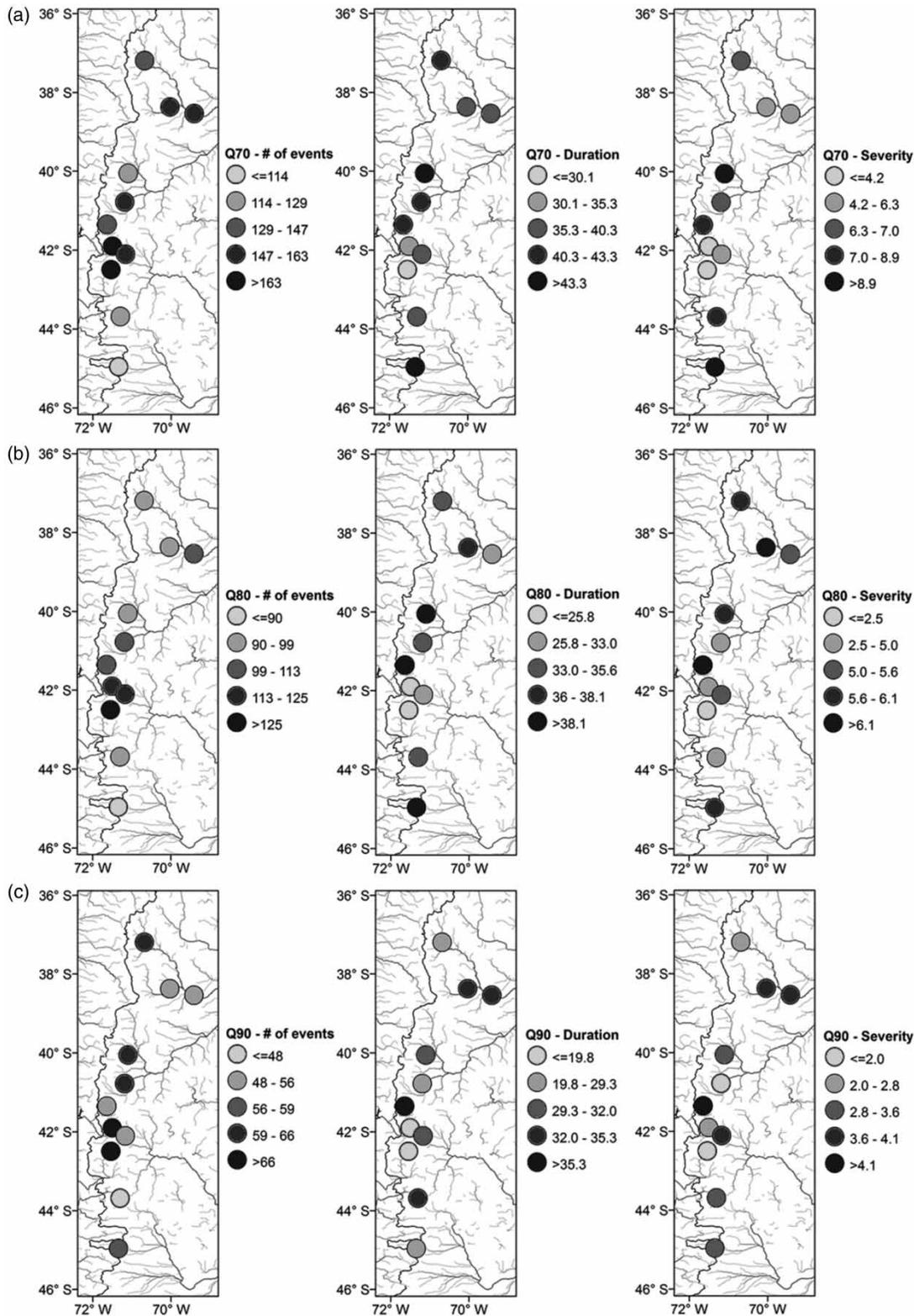
**Figure 2** | Streamflow drought indicators for the stations selected for the climatological assessment: (left panel) number of drought events in the period 1962/63–2014/15, (center panel) mean drought duration (in days), and (right panel) mean drought severity (in days) for (a) Q70, (b) Q80, and (c) Q90 thresholds.
