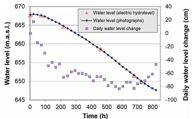
**Figure 9** | Evolution of reservoir water level obtained from measurements in photos and daily descents, obtained by difference of each day with respect to the previous day.
