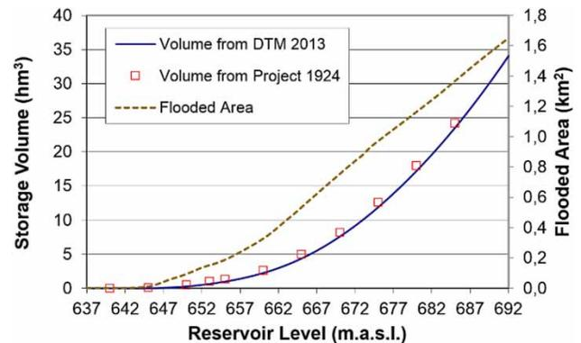
**Figure 8** | Results obtained from the DTM analysis of the reservoir basin: graphs of flooded area and stored volume versus reservoir water level and comparison with historical data.
