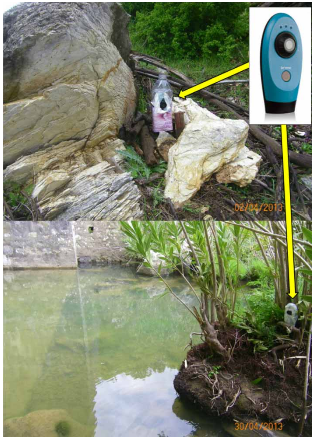
Figure 5 | Brinno-TLC100 camera hidden in the ground at a location near the dam (above) and near the river, where it flows into the reservoir (bottom).
