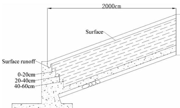
**Figure 2** | Profile of the runoff plot.
