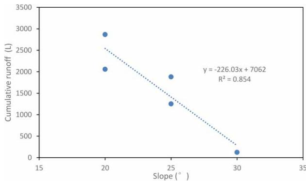
**Figure 8** | Fitting curve of cumulative runoff and slope.
