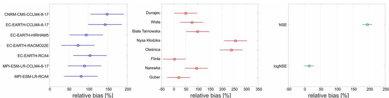
**Figure 8** | Quantification of the spread in the results (biases in volume deficit) due to differences between climate models, catchments and objective functions. Circles represent the PMM and the bars are the relevant spread.
