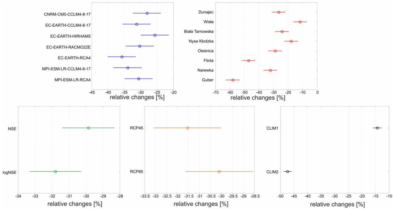
**Figure 11** | Distribution of relative changes in the number of days under threshold (Q80) as a function of climate model, catchment, objective function, emission scenario and future period based on five-way ANOVA and Tukey post-hoc test. Circles represent the PMM and the bars are the relevant spread.
