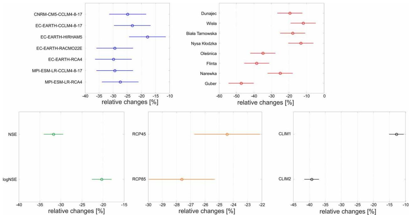
**Figure 12** | Distribution of relative changes in the mean duration of low flow events as a function of climate model, catchment, objective function, emission scenario and future period based on five-way ANOVA and Tukey test. Circles represent the PMM and the bars are the relevant spread.
