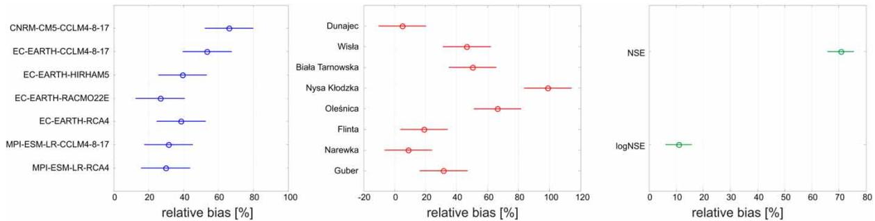
**Figure 6** | Quantification of the spread in the results (biases in the number of days below threshold) due to differences between climate models, catchments and objective functions. Circles represent the PMM and the bars are the relevant spread.
