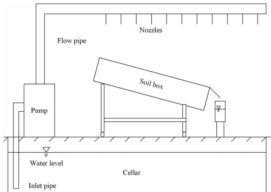
**Figure 1** | The schematic diagram of the rainfall simulator.
