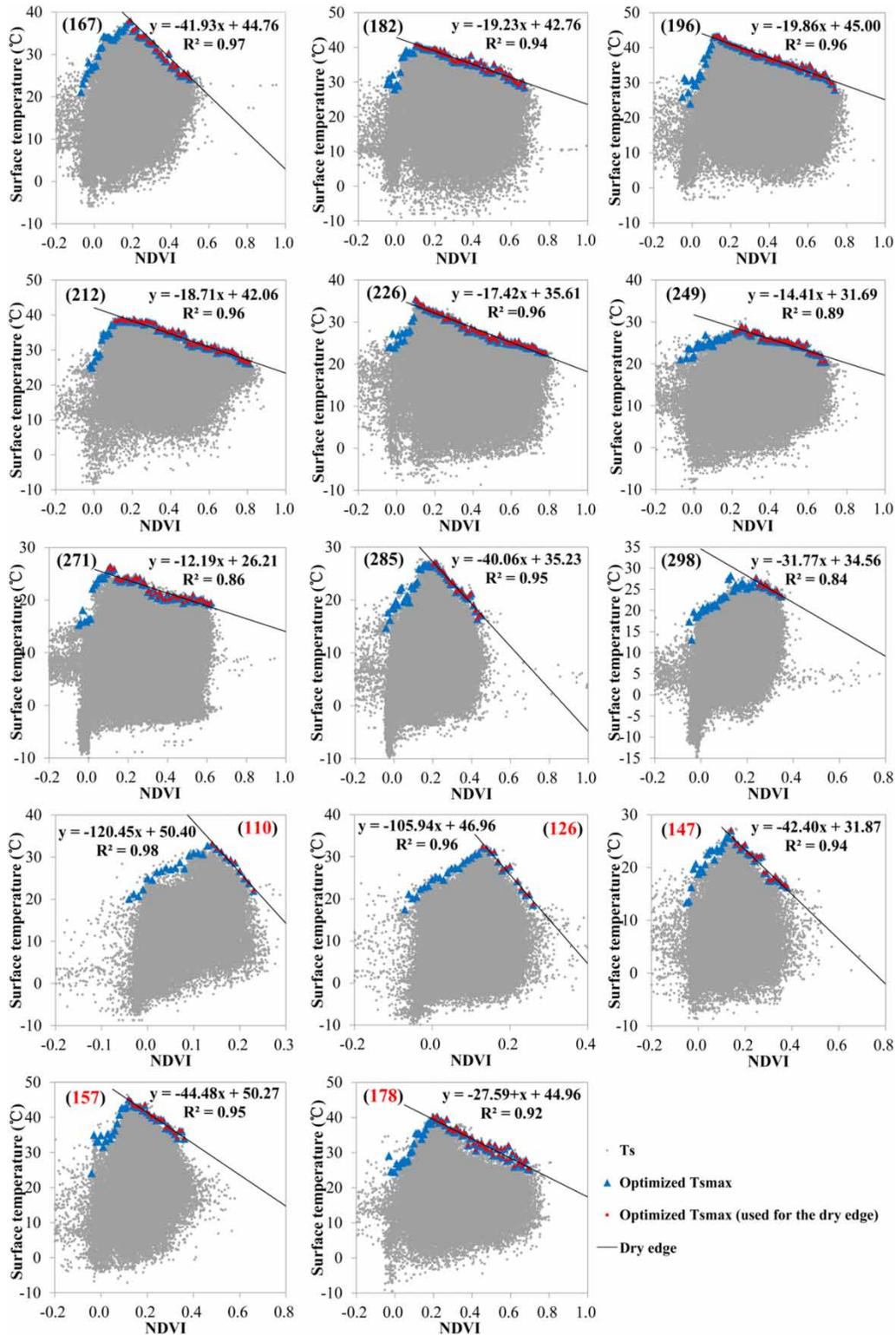
**Figure 4** | Normalized  $T_s$ -NDVI scatter plots and dry edges. The triangle denotes the optimized maximum  $T_s$  in each bin of the NDVI. The dot is the optimized maximum  $T_s$  used for dry edge extraction. The line indicates the dry edge. The first nine plots are observations during 2014, while the last five plots are observations during 2015.
