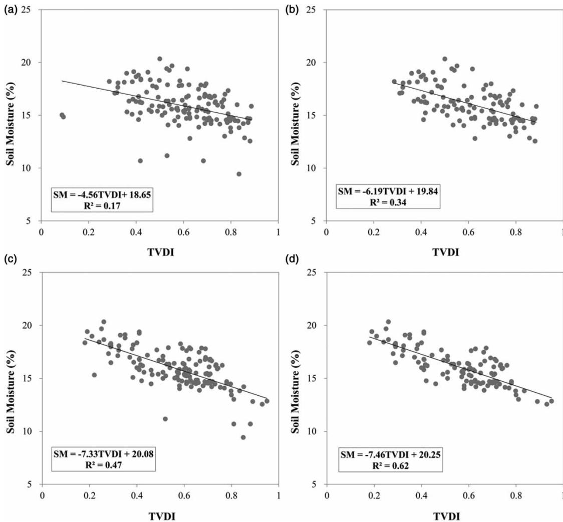
**Figure 6** | Scatter plots of TVDI and observed SSM when: (a) not considering the effects of altitude or frozen soil; (b) considering the effect of frozen soil only; (c) considering the effect of altitude only; and (d) considering the effects of both altitude and frozen soil.
