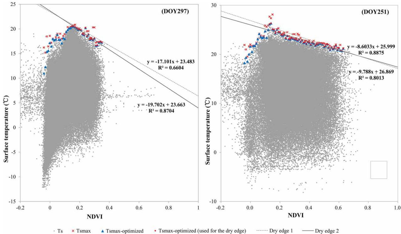
**Figure 2** | Schematic diagram illustrating the optimized dry edge.
