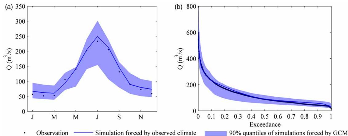
**Figure 3** | Observed (dots) and simulated streamflows forced by the observed meteorological data (lines) and bias-corrected GCM outputs (shaded area representing 90% percentile) for the control period: (a) monthly average streamflows and (b) exceedance probability curve of the streamflows.
