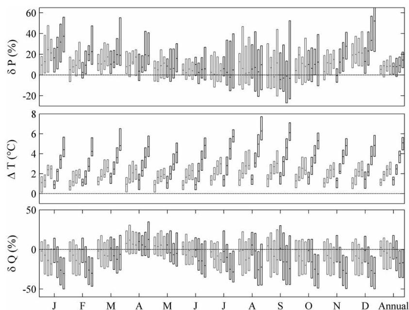
**Figure 4** | GCM projected monthly precipitation change ( $\delta P$ ), temperature change ( $\Delta T$ ) at the Bayanbulak station, and projected streamflow change ( $\delta Q$ ) under RCP4.5 (grey) and RCP8.5 (black) for the four periods in the 21st century (four boxes sequentially).
