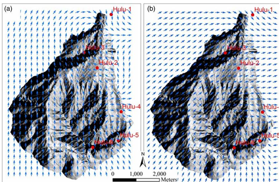
**Figure 9** | Wind field at 1.5 m height at 8:30 (a) and 15:30 (b) on July 14, 2015, in the Hulu watershed. Wind direction is interpolated with data at Hulu-1-6 stations.
