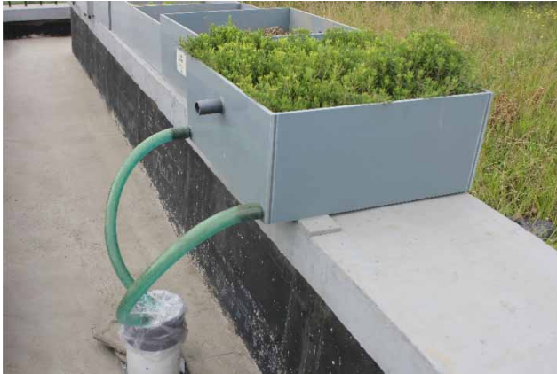
Figure 2 | An example experimental EGR module having Sedum lineare Thunb, drainage pipes and a rain gauge.
