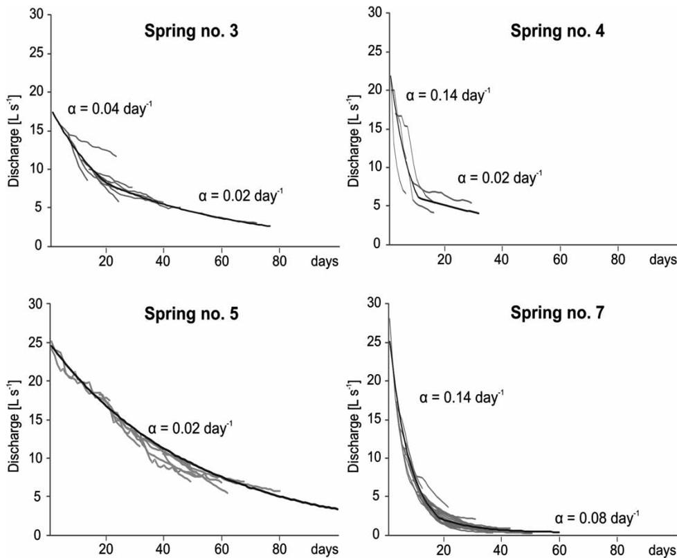
**Figure 4** | Master recession curves of the studied springs.
