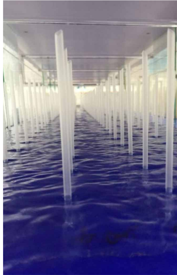
Figure 1 | Showing the farmland vegetation row direction, and water flow directions with different flow angles.
