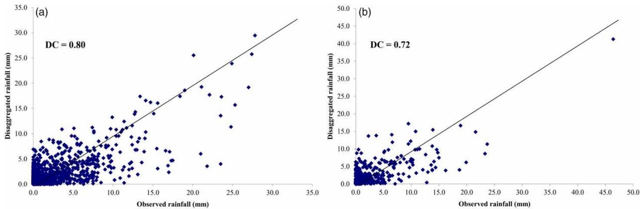
**Figure 6** | Scatter plot of observed versus disaggregated rainfall (in mm) using WANN at Tabriz station for (a) calibration period, (b) verification period.
