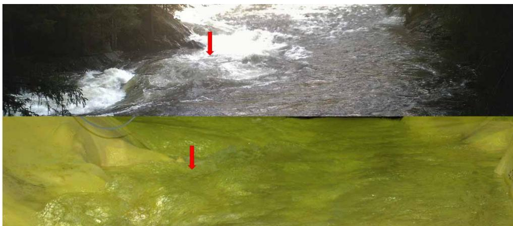
**Figure 5** | Flow at  $\sim 200 \text{ m}^3/\text{s}$  in the field (top) and the hydraulic scale model (bottom). The arrows indicate the location of point GS. Flow direction from the top towards the bottom.
