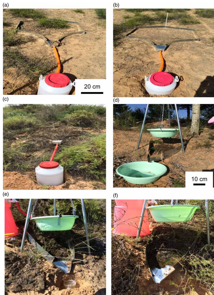
Figure 2 | Natural rainfall experiments for the bare land (a), lichen- (b) and moss-dominated biocrusts (c) and artificial rainfall experiments for the bare land (d), lichen- (e) and moss-dominated biocrusts (f).
