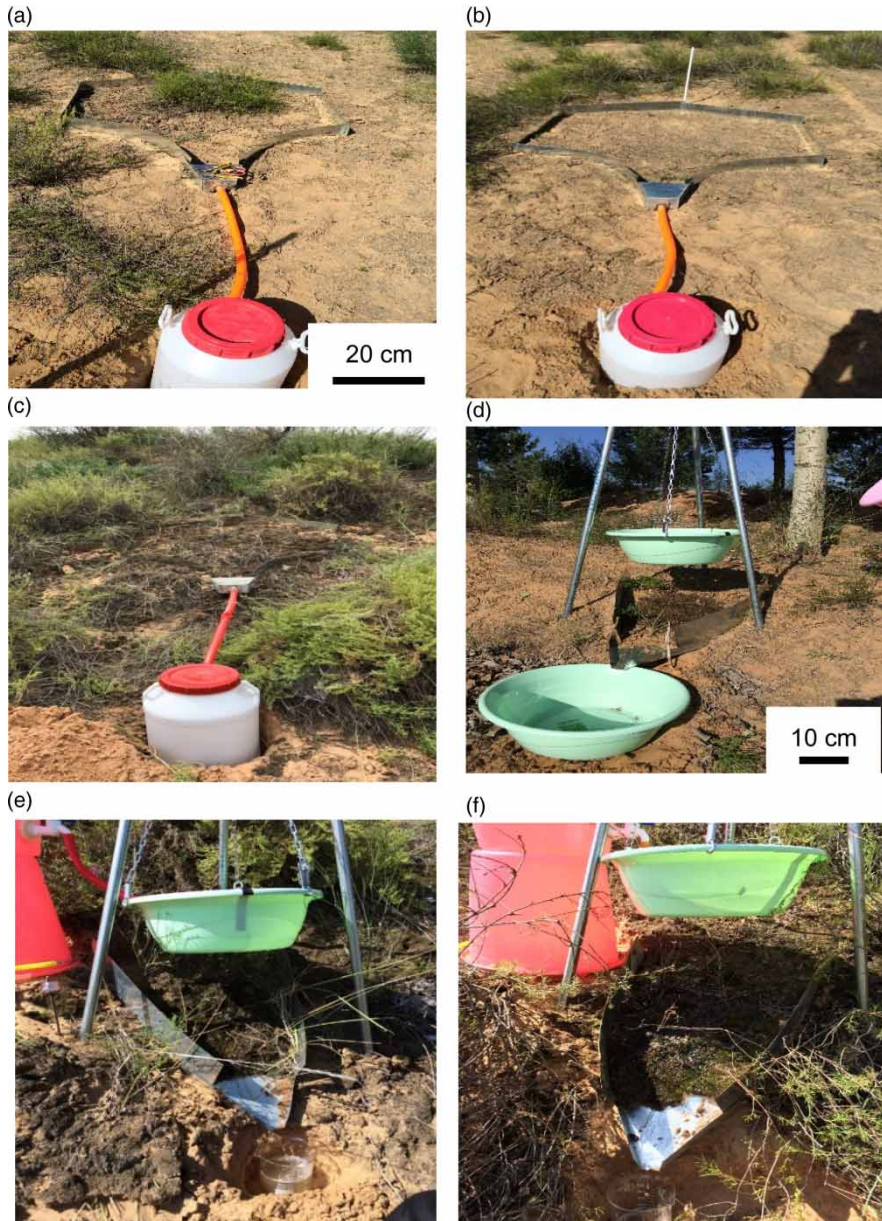
Figure 2 | Natural rainfall experiments for the bare land (a), lichen- (b) and moss-dominated biocrusts (c) and artificial rainfall experiments for the bare land (d), lichen- (e) and moss-dominated biocrusts (f).
