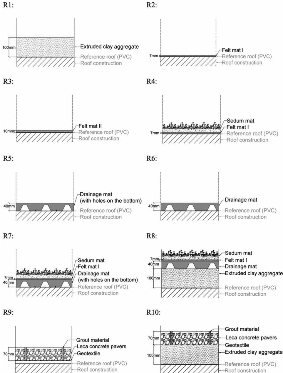
**Figure 1** | Section drawings for the composition of the different runs; R#.
