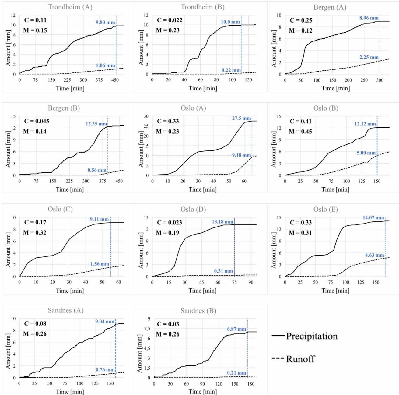
**Figure 6** | Precipitation and runoff curves for the chosen field events, runoff coefficient ( $C$ ) and moisture ( $M$ ) at the start of precipitation. The blue represents the values used in the calculation of the runoff coefficient. Please refer to the online version of this paper to see this figure in colour: <http://dx.doi.org/10.2166/nh.2020.049>.
