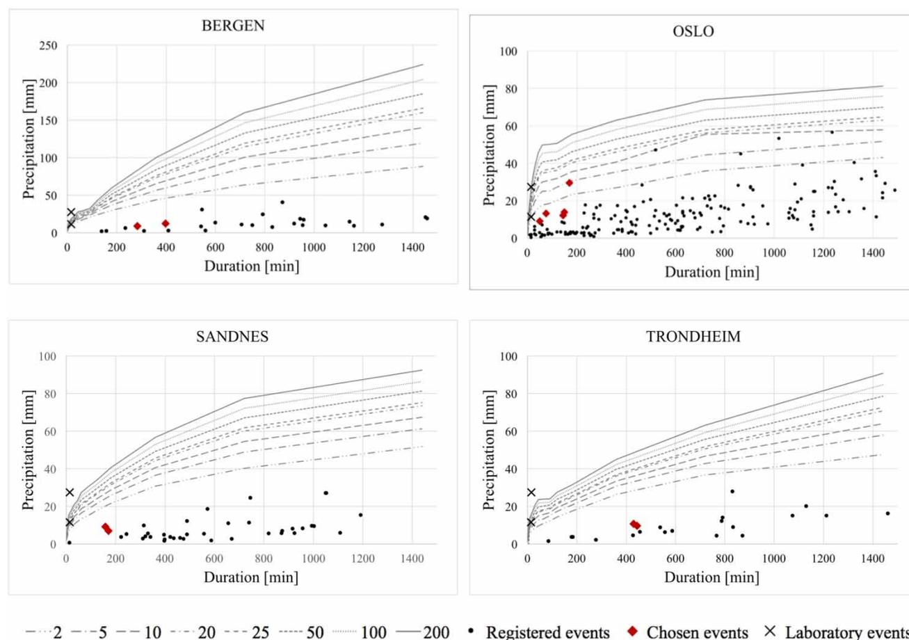
**Figure 3** | IDF curves and precipitation events from the field measurements, where X for laboratory events includes both the FLL prescribed precipitation event of 27 mm/15 min and the 11.4 mm/15 min selected based on the field locations.
