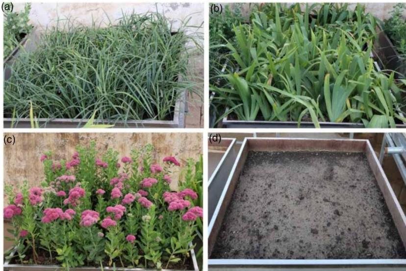
**Figure 2** | Runoff plots of green roofs in the field experiment. (Note: The letters a, b, c and d represent green roof GR-5, GI-10, GS-15 and BG-5, respectively).
