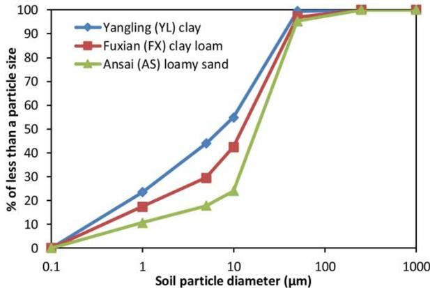
Figure 1 | Particle size distributions for tested soils.
