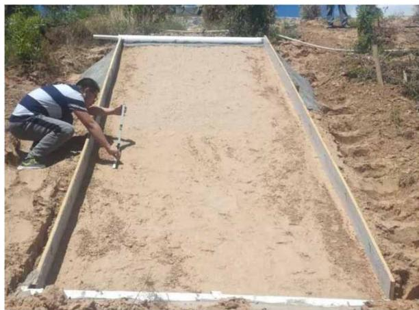
**Figure 2** | Field runoff plot system at the study site.
