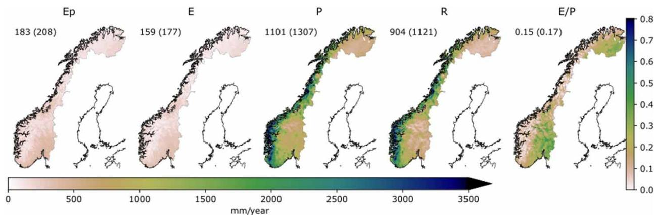
**Figure 6** | The 1980–2014 mean annual potential evaporation ( $E_p$ ), evaporation ( $E$ ), precipitation ( $P$ ), runoff ( $R$ ), and  $E/P$ , in mm/year. The areal median and mean are denoted in the upper left corner, with the mean in parenthesis. Please refer to the online version of this paper to see this figure in color: <https://doi.org/10.2166/nh.2021.132>.
