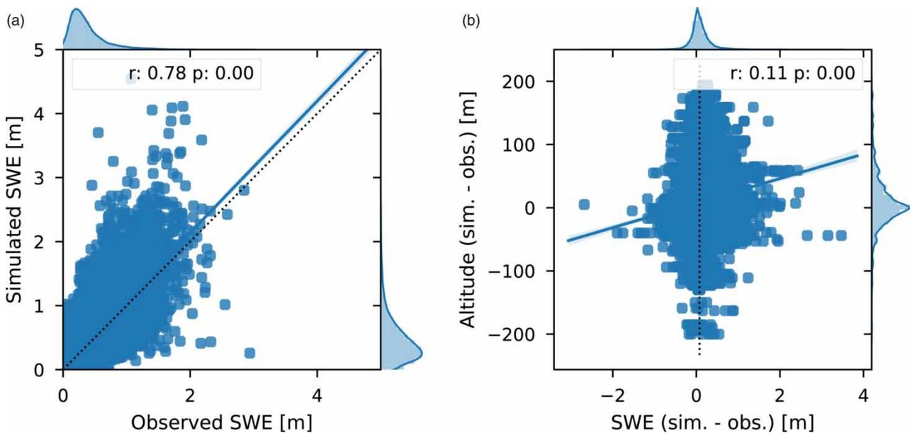
**Figure 3** | Observed (x) and simulated (y) SWE around the time of maximum SWE (a), and difference between simulated and observed SWE (x) plotted against difference in altitude between the model grid cell and observation (y) (b). The Pearson correlation and its significance are denoted near the top of each plot.
