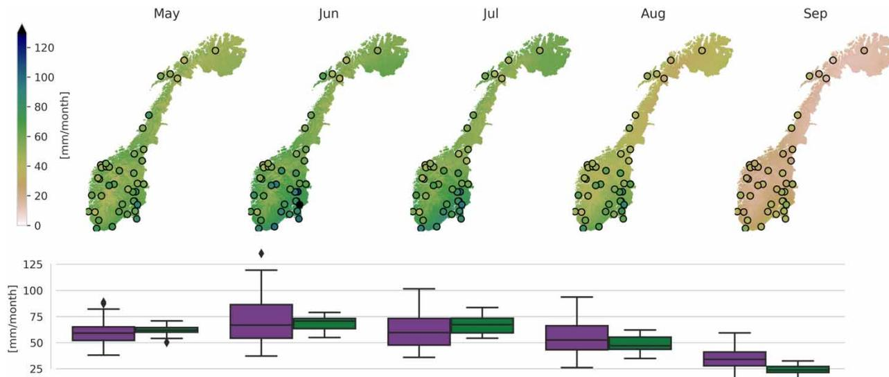
**Figure 4** | Mean monthly pan evaporation measured at 42 sites across Norway (1967–1972) shown within black circles overlaid the simulated  $E_p$  for the land cover class ‘Open’ (1979–1984). The lower box plots show the pan measurements in purple and the simulated  $E_p$  for collocated grid cells in green. Please refer to the online version of this paper to see this figure in color: <https://doi.org/10.2166/nh.2021.132>.
