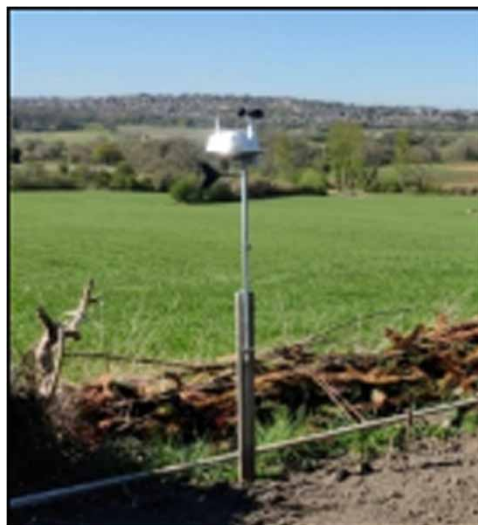
Figure 1 | Photograph showing a citizen science rain gauge in situ .
