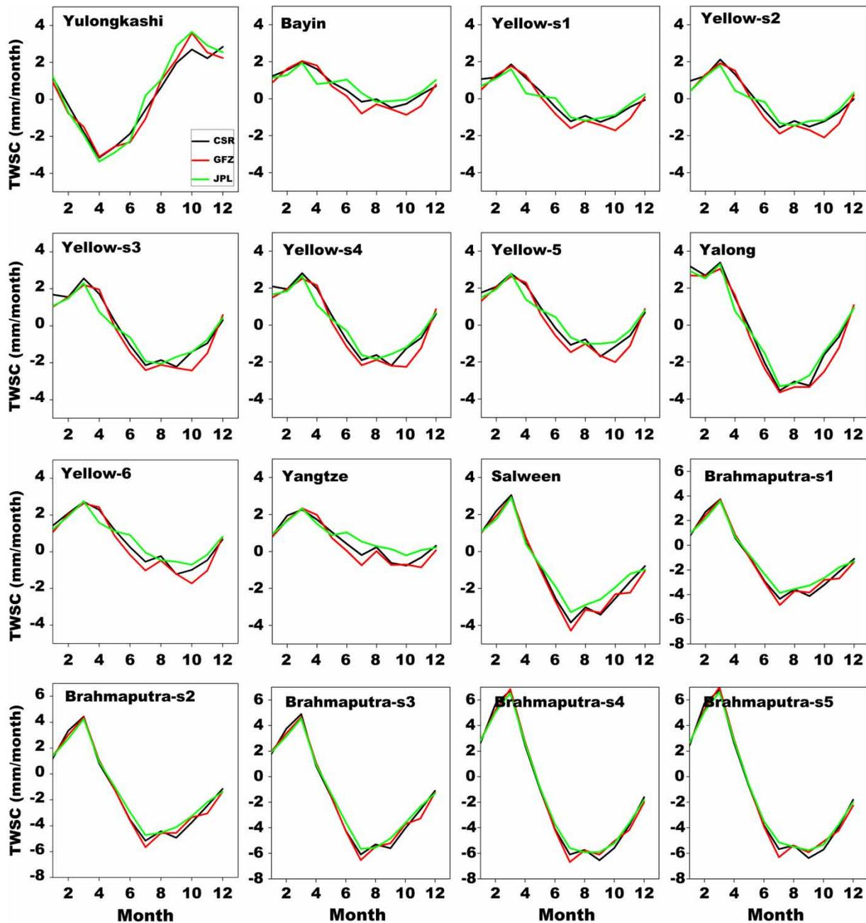
Figure 6 | Comparison of GRACE-derived terrestrial water storage changes (TWSC) processed at CSR, JPL and GFZ.
