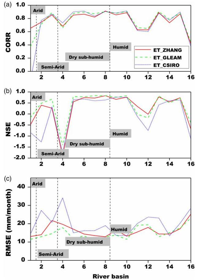
**Figure 4** | Comparison of Spearman's rank correlation coefficient (a) Nash-Sutcliffe efficiency (*NSE*) (b) and root-mean-square-error (*RMSE*) (c) of monthly remotely sensed ET products against water balance-based ET in 16 TP basins. The basins are classified into four classes based on the aridity index ( $AI = \text{precipitation}/\text{potential evaporation}$ ), i.e., arid ( $0.03 < AI < 0.2$ ), semi-arid ( $0.2 < AI < 0.5$ ), dry sub-humid ( $0.5 < AI < 0.65$ ) and humid ( $AI > 0.65$ ).
