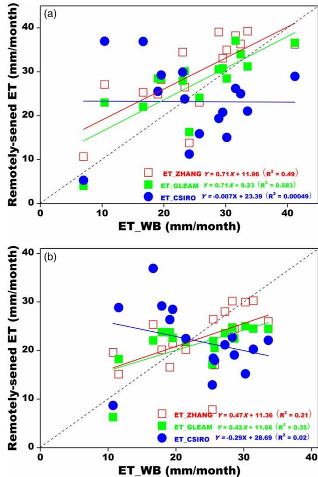
**Figure 2** | Comparison of the multi-year average (a) and the standard deviation (b) of monthly remotely sensed and water balance-estimated ET in 16 TP basins.
