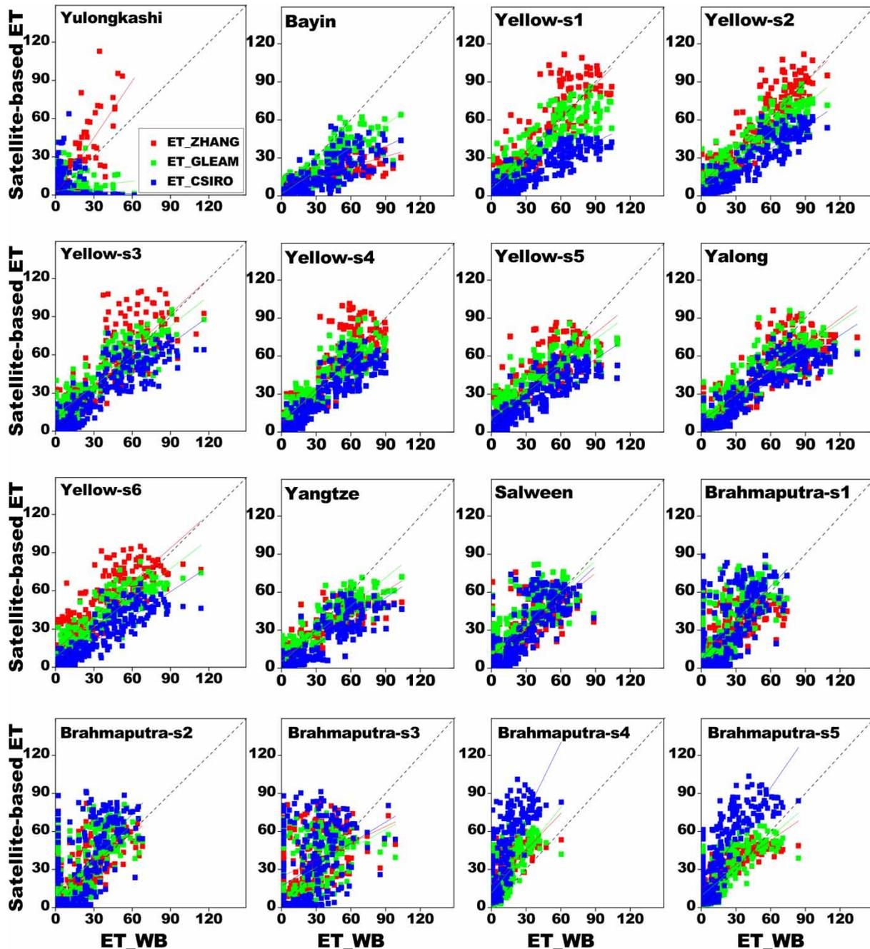
**Figure 3** | Validation of three satellite-based monthly ET measurements against water balance estimates ( $ET_{WB}$ , mm/month) in 16 TP river basins during the period of 1983–2011.
