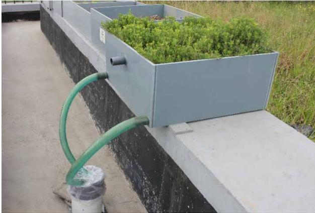
**Figure 2** | An example experimental EGR module having Sedum linearis Thunb, drainage pipes and a rain gauge.
