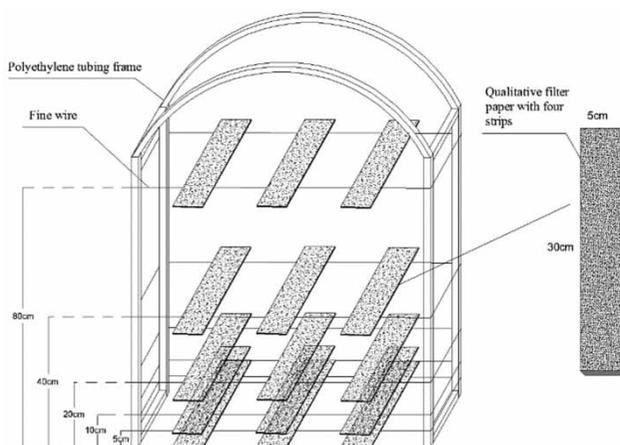
**Figure 1** | Dew collection device using simulated condensation surface.
