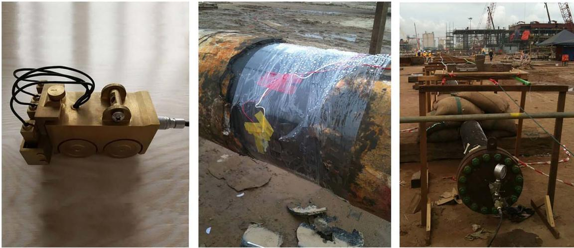
**Fig. 3 Magnetic measurement instrument and experimental setup with strain gage installation and internal pressure measurement (based on the work of Dr. Sheng Bao)**
