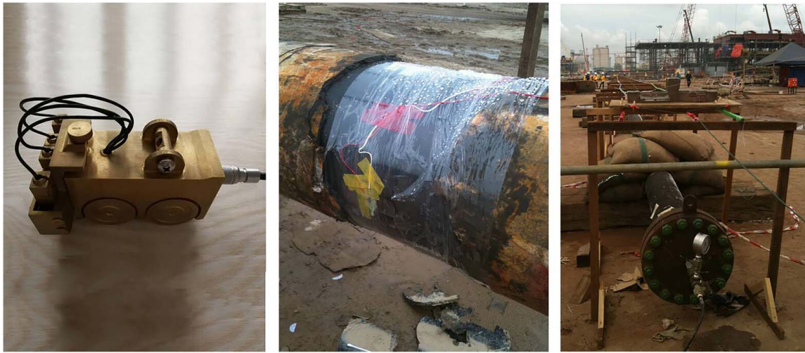
Fig. 3 Magnetic measurement instrument and experimental setup with strain gage installation and internal pressure measurement (based on the work of Dr. Sheng Bao)
