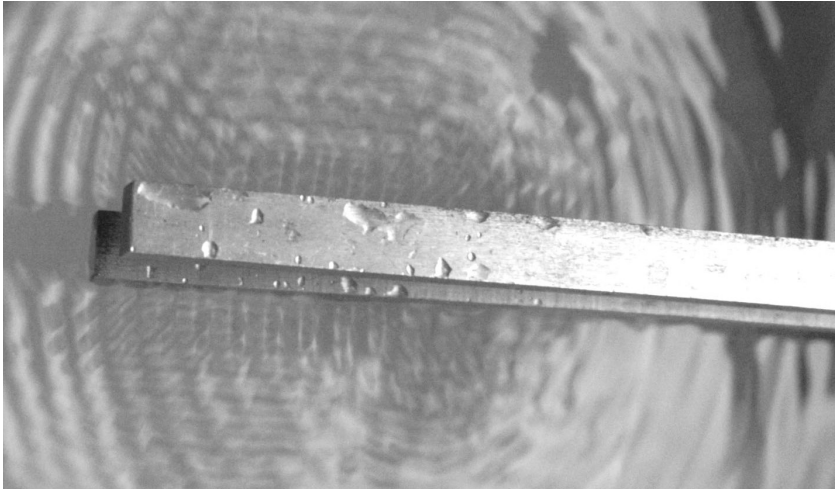
Figure 6. Ridge waves appear in water, perpendicular to the tuning fork's tines. Photo by James Bales, MIT Edgerton Center, using a Nikon D-100 at a shutter speed 1/160s, f6.3, focal length 40mm.
