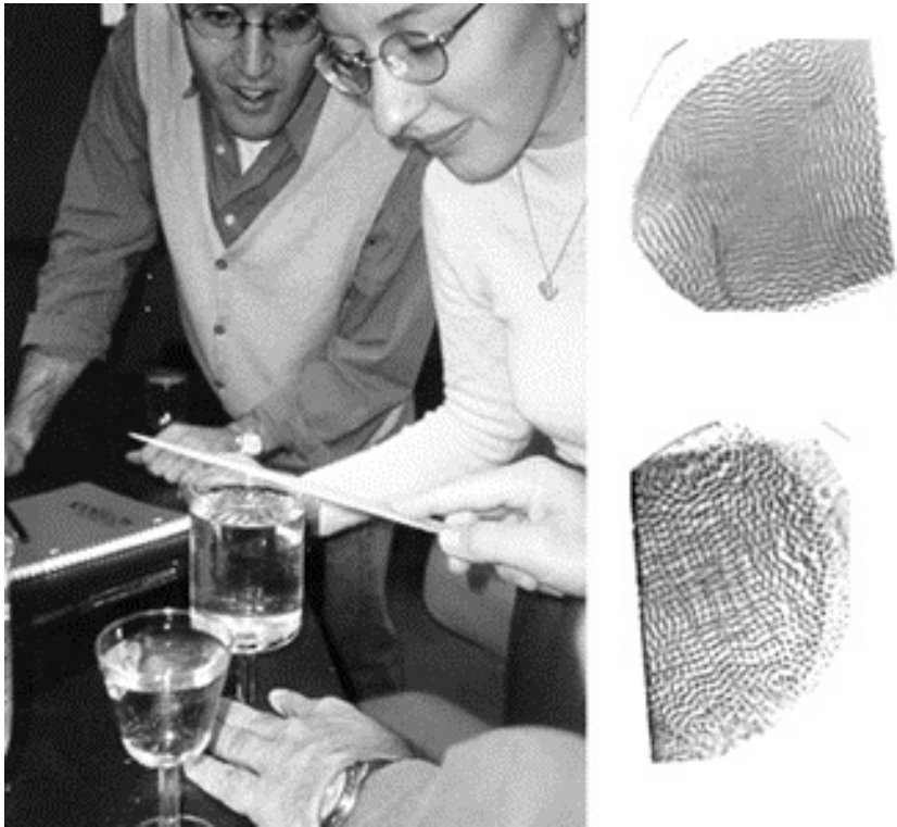
Figure 3. Left: Two teachers watch while another teacher vibrates a water glass with the teeth of a wood rasp. Right: Two photograms showing crispations produced when a wineglass was vibrated by a string bass bow (November 29, 1999).
