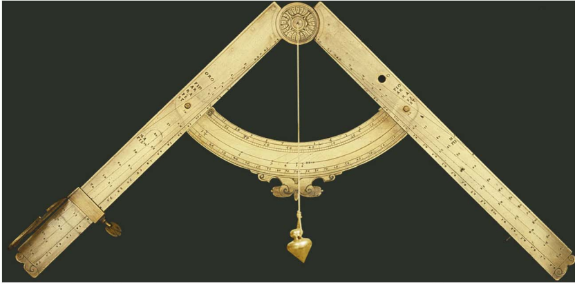
Figure 2. Galileo's compass set up as a gunner's squadra . Image used with permission of the Collection of Historical Scientific Instruments, Harvard University.
