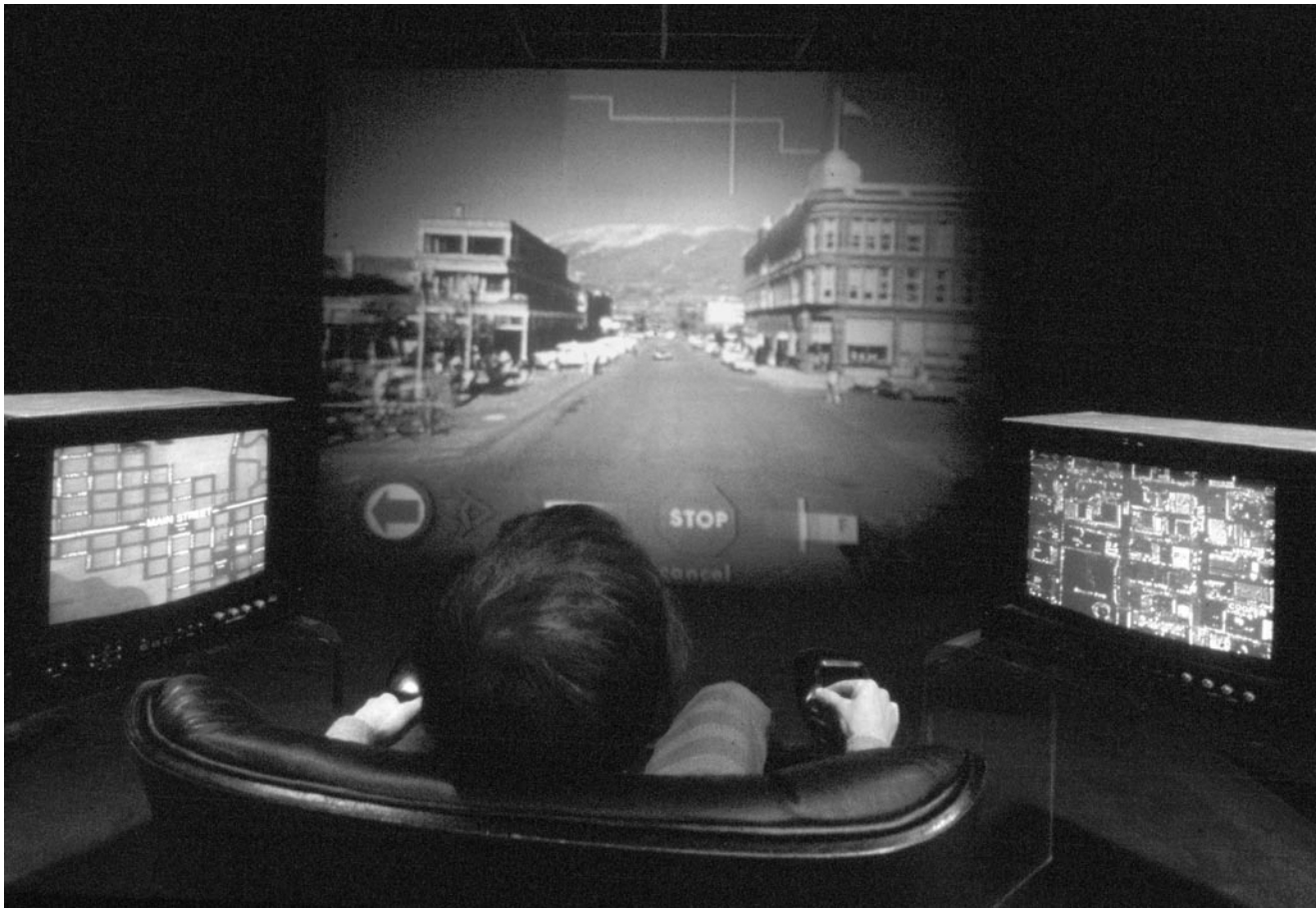
Figure 1. The Aspen Moviemap experienced in the “Media Room” at the Architecture Machine Group, MIT, c1980. The “traveler,” seated in an instrumented armchair, controls speed and direction of travel. Touch screens displaying map and aerial views allow access to additional multimedia material. (Photo: Bob Mohl.)
