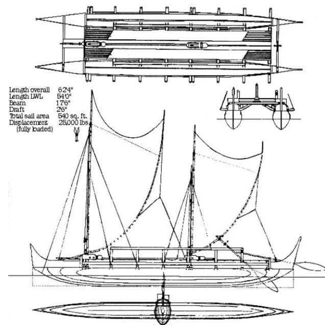
**Figure 1.** Original construction drawings for the Hōkūle‘a. From “Founding the Polynesian Voyaging Society; Building Hōkūle‘a,” by Ben Finney ([http://archive.hokulea.com/like/kalai\\_waal/finney\\_building\\_hokulea.html](http://archive.hokulea.com/like/kalai_waal/finney_building_hokulea.html)). © Polynesian Voyaging Society, reprinted with permission.
