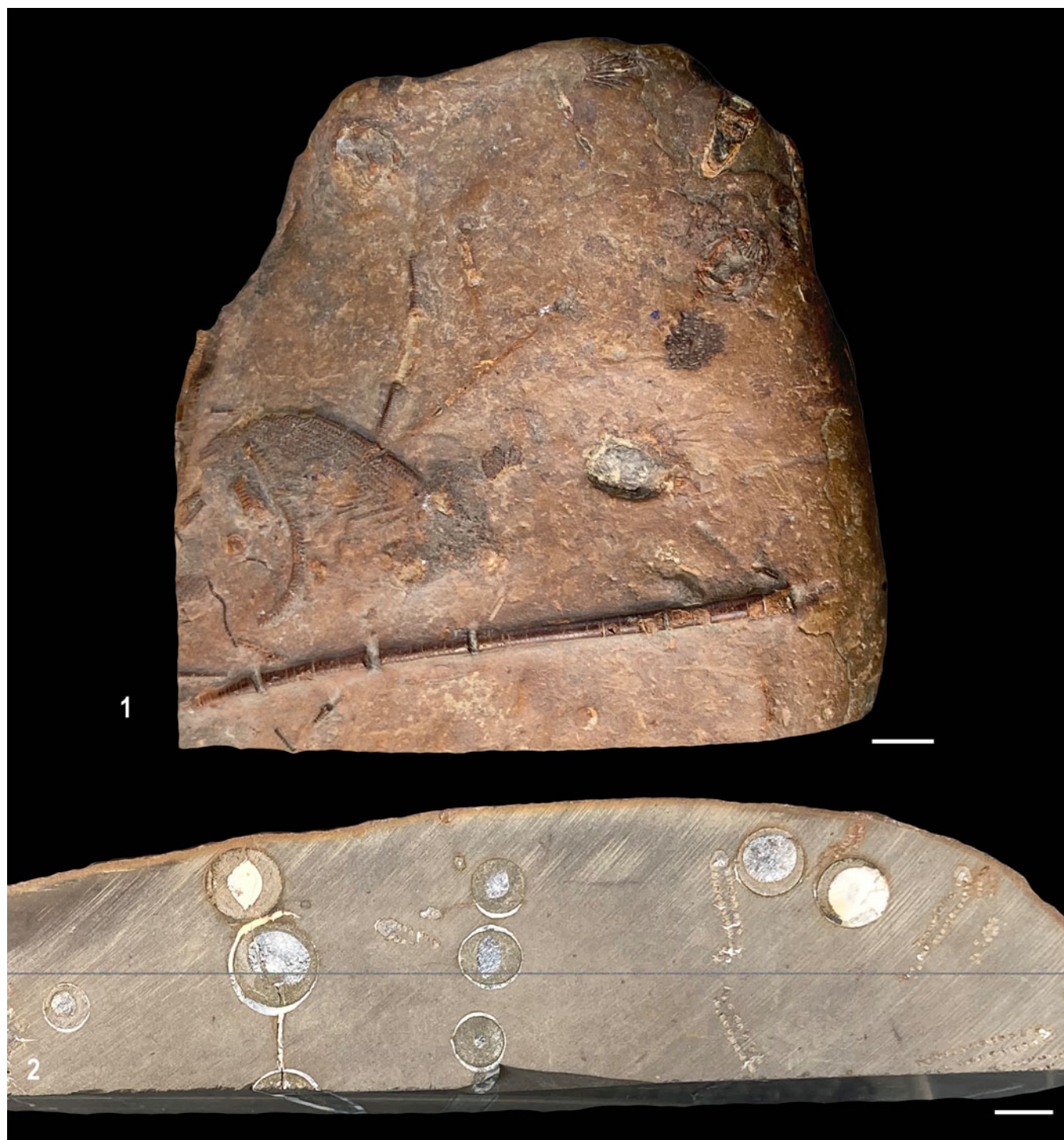
Figure 7. CMNH 18019 bed largely replaced by siderite (white is calcite). (1) Upper part of bedding surface completely replaced; (2) cross section through bed illustrating various modes of replacement of columnals with siderite; note infilling of fractures with calcite; bed is slightly tilted to illustrate that the pattern of replacement on the cross section continues into the bed. Scale bar represents 5.0 mm in (2), 10.0 mm in (1).
