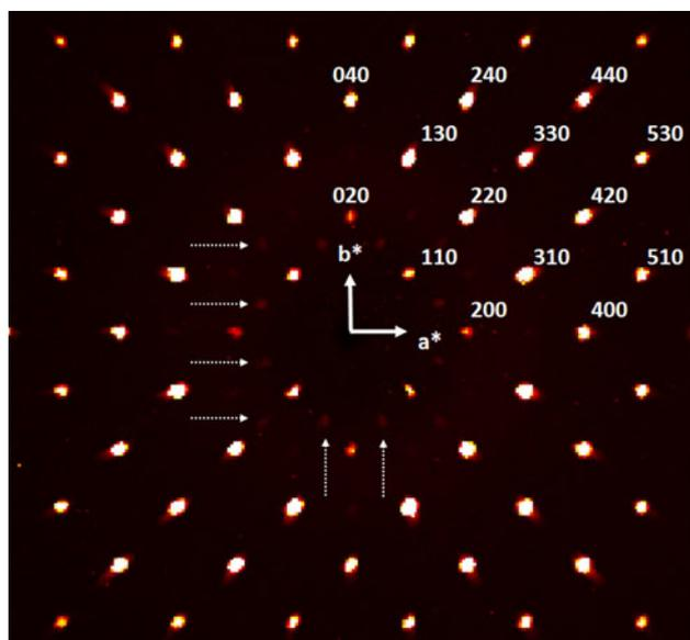
**Fig. 3.** Reconstructed precession image of the  $hk0$  reciprocal lattice plane. Weak not-indexed reflections at lower angles can be observed (some of them are indicated by thin dotted arrows). Only positive  $h$  and  $k$  indices are shown.
