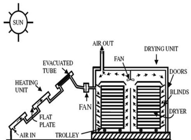
**Fig. 14 Hybrid solar dryer [50]**
