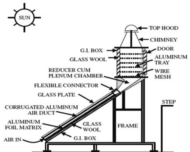
Fig. 7 Multipurpose natural convection solar dryer [34]
