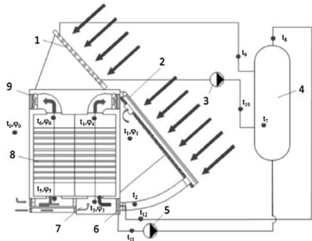
**Fig. 13 Basic scheme of the dryer for medicinal plants: (1) flat-plate type solar collector (8 m<sup>2</sup> area), (2) air-type solar collector (12 m<sup>2</sup> area), (3) and (5) a pump, (4) a tank with water for heat storage, (6) heat exchanger, (7) air mixing chamber, (8) drying chambers, and (9) fan [49]**
