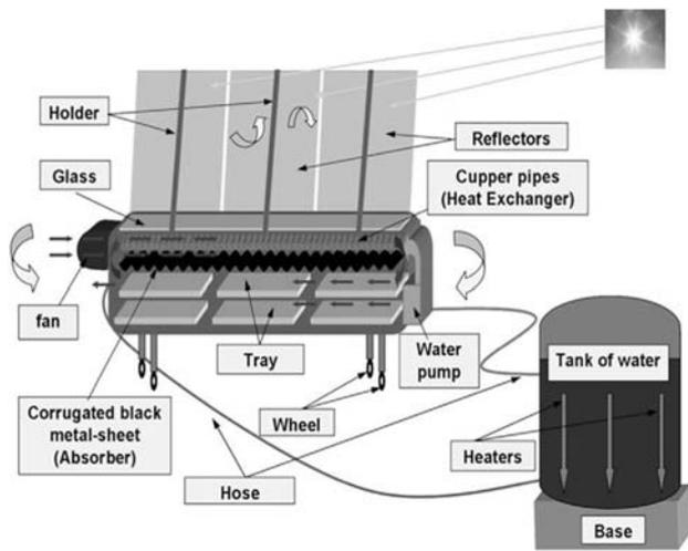
Fig. 4 Schematic diagram of a hybrid solar dryer [54]
