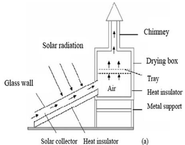
Fig. 2 Indirect solar dryer [6]
