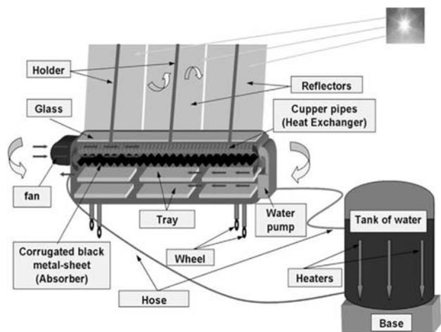
**Fig. 16 Schematic diagram of a solar hybrid dryer [61]**
