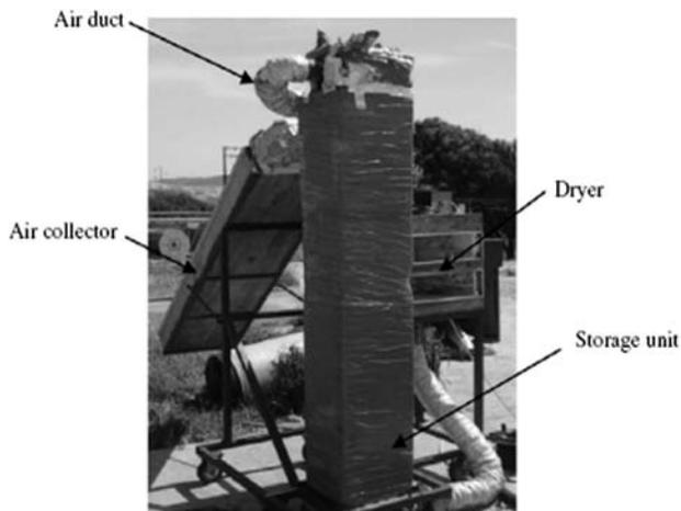
Fig. 19 Photograph of the drying solar unit [76]
