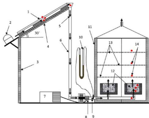
**Fig. 18 Schematic diagram of the experimental setup: (1) solar air heater, (2) pyranometer, (3) the room wall, (4) the room roof, (5) flowing air, (6) PVC tube, (7) inverter, (8) three-phase induction motor coupled with fan, (9) pilot tube, (10) U tube manometer, (11) drying compartment, (12) PCM, (13) trays, and (14) thermocouple positions [69]**
