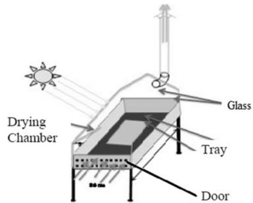
Fig. 1 Direct solar dryer [3]
