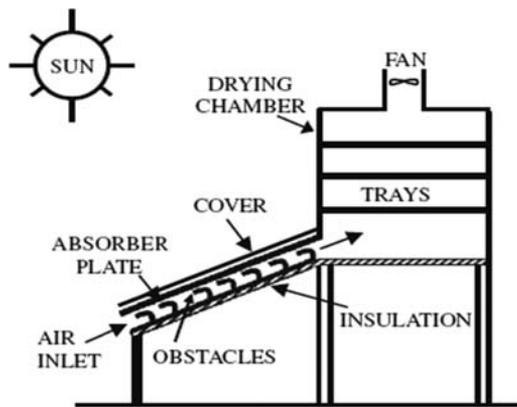
Fig. 8 Solar air collector with obstacles [35]
