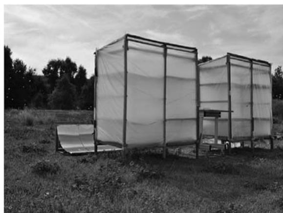
Fig. 11 Dryer 2 (left) is exposed to the concave solar concentrator, and dryer 1 (right) is the control [43]
