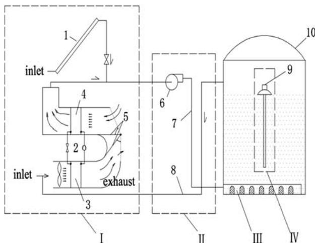
**Fig. 12 Schematic diagram of the solar-assisted heat pump in-store drying system: (1) solar air collector, (2) air source heat pump, (3) evaporator, (4) condenser, (5) movable diaphragm, (6) supply fan, (7) ventilation supply tube, (8) air recycle tube, (9) grain stirrer, and (10) granary [47]**
