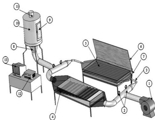
**Fig. 17 Schematic view of the manufactured experimental setup: (1) fan, (2) valves, (3) connection pipe, (4) expanded surface solar air collector, (5) collector with PCM, (6) adjustable mirror, (7) adjustable collector tripod, (8) diffuser, (9) observation glass, (10) drying room, (11) air exit chimney, (12) data logger, and (13) PC [66]**
