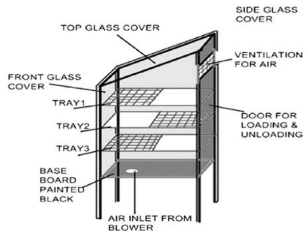
Fig. 3 Mixed-mode solar dryer [8]
