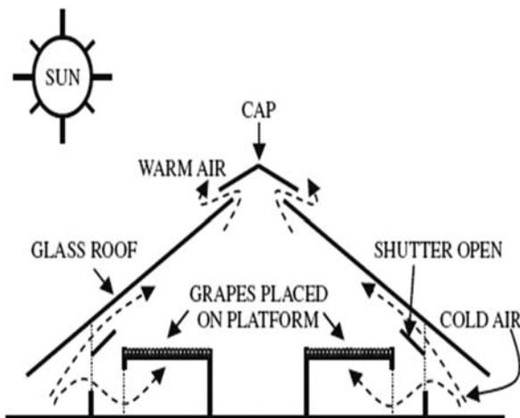
Fig. 5 Glass roof solar dryer [32]
