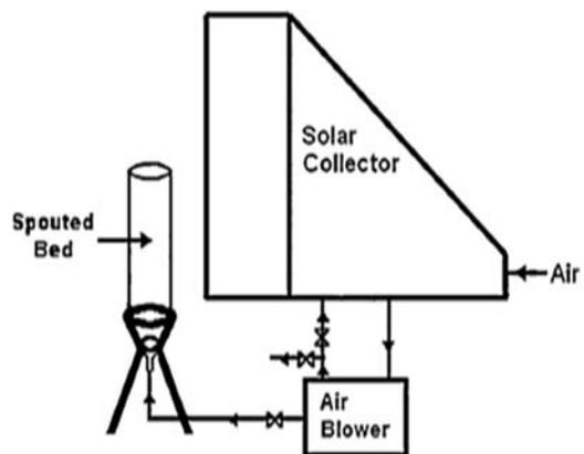
Fig. 10 Schematic diagram of a solar-spouted bed dryer [37]
