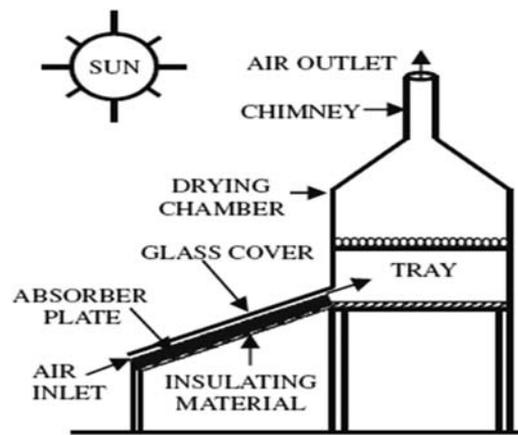
Fig. 6 Indirect natural convection solar dryer with chimney [33]
