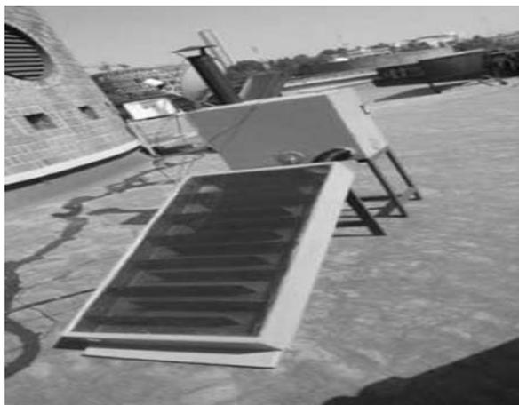
Fig. 9 Indirect solar dryer with variable steering flow [36]
