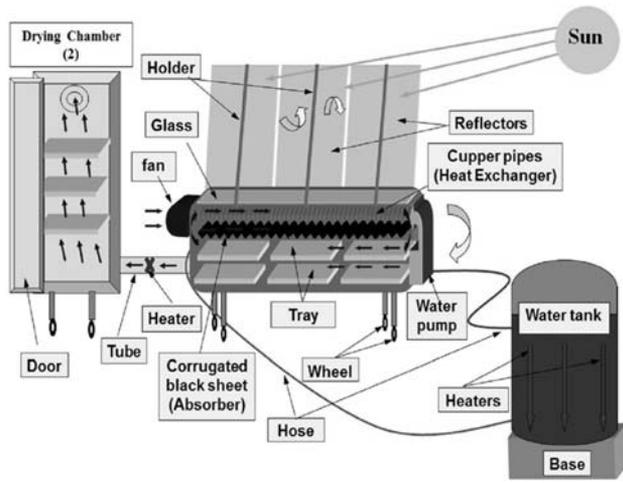
**Fig. 15 Schematic diagram of the components of the integrated solar dryer system [51]**
