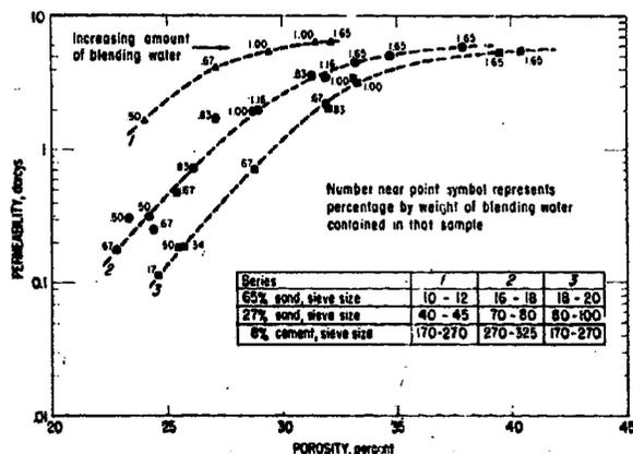
FIG. 1 — RELATIONSHIP OF PERMEABILITY TO POROSITY FOR SEVERAL GRAIN-SIZE COMBINATIONS AND BLENDING WATER CONTENT.
