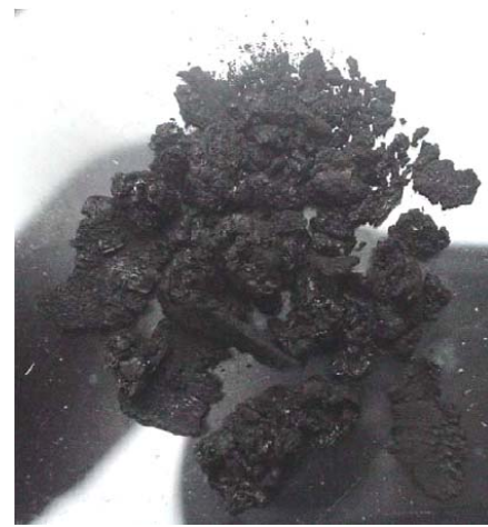
Figure 2. Picture showing organic residues collected from production tubing in a Ceuta field well.
